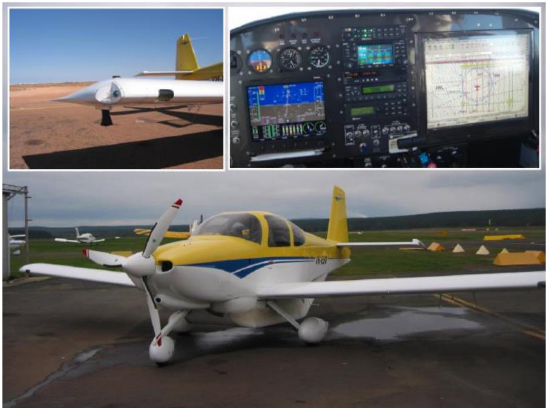
Fig. 1. Aircraft for remote sensing experiments, showing a wingtip installation in the left inset, and the cockpit with cockpit computer display in the right inset.
